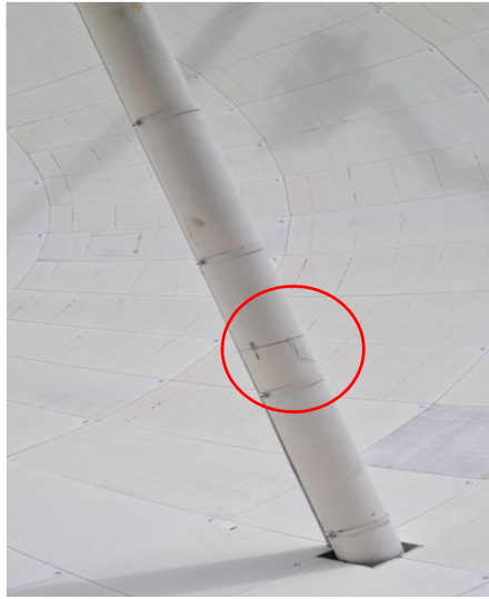
Figure 1: Detail of a thermal sensor in one of the tetrapod legs.
