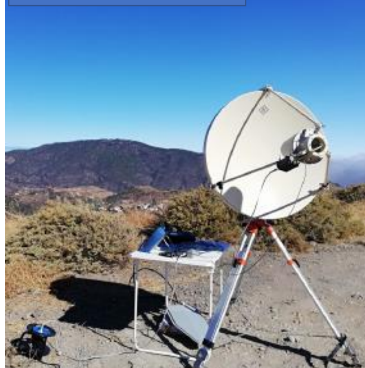
Portable RFI system Santa María (Azores, Portugal), Gran Canaria (Spain)
