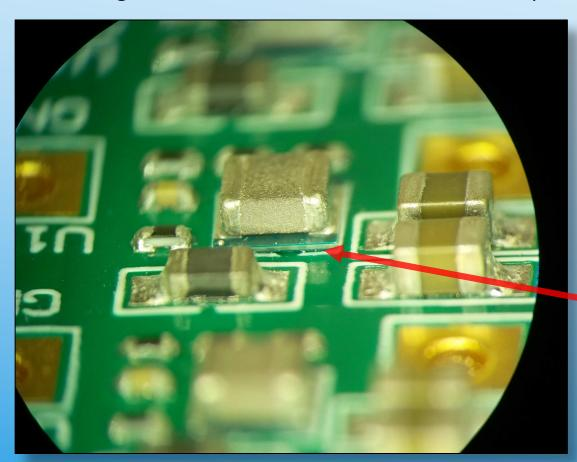
Tilted power-regulators due to uneven solder mask surface
