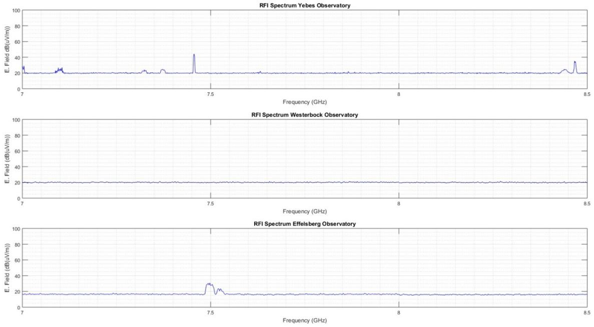
Figure 9: 7 - 8.5 GHz RFI spectrum comparison.
