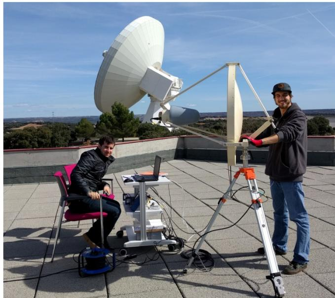
**Figure 2: RFI measurements on the roof of Yebes laboratory building.**
