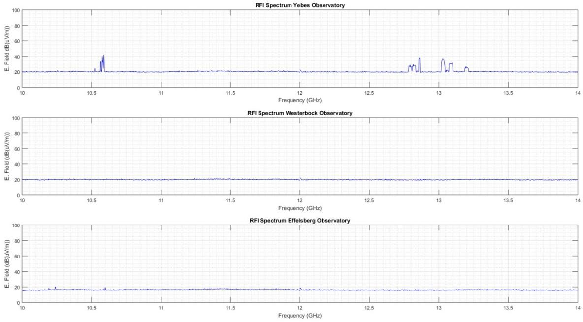
Figure 11: 10 - 14 GHz RFI spectrum comparison.
