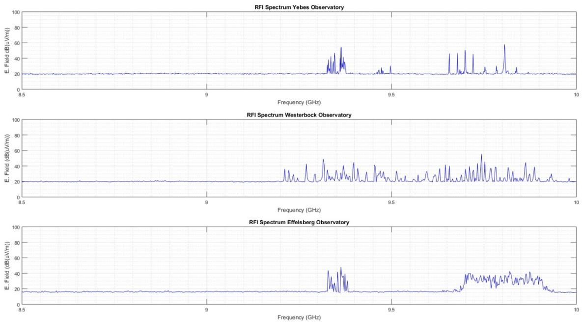
Figure 10: 8.5 - 10 GHz RFI spectrum comparison.
