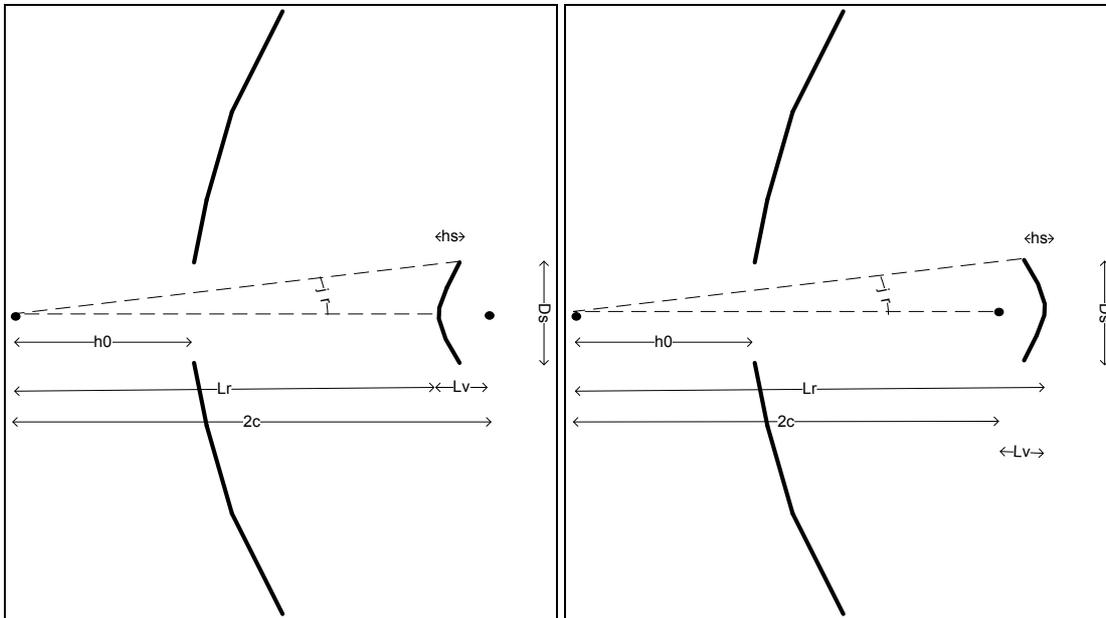
Figure 2. Cassegrain and Gregorian SECONDARY parameters
