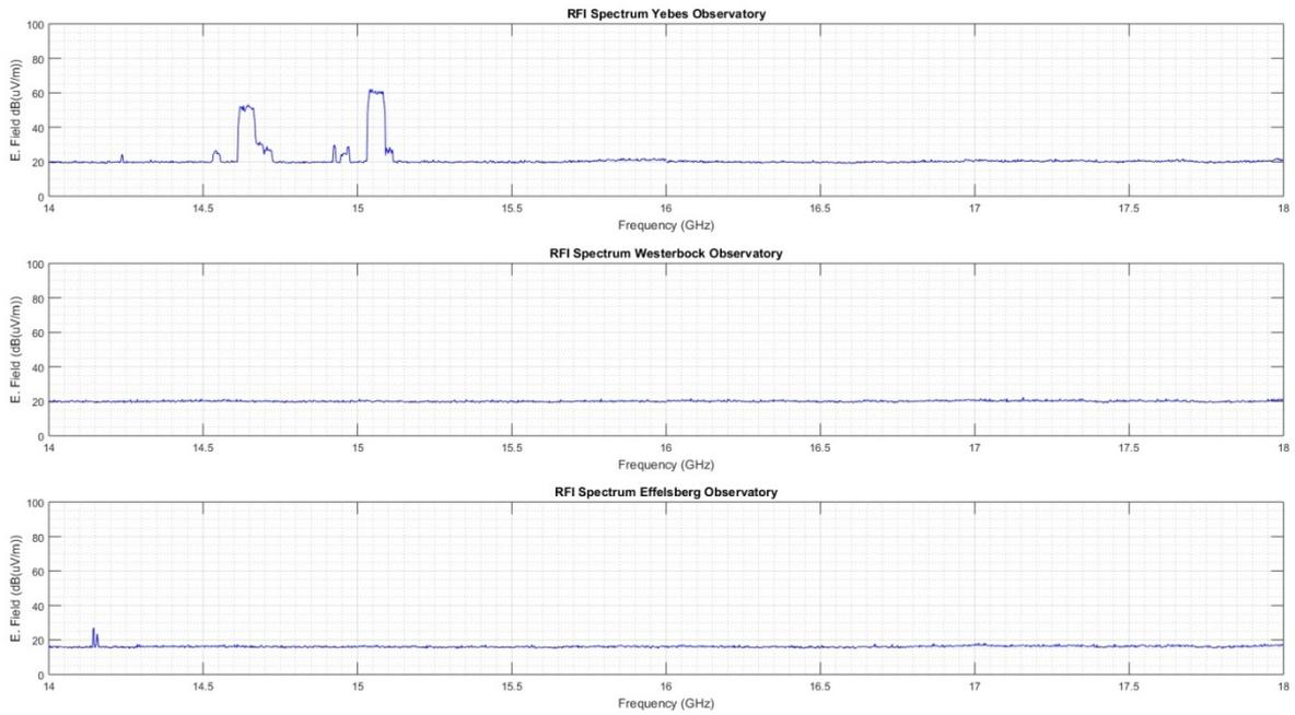
Figure 12: 14 - 18 GHz RFI spectrum comparison.
