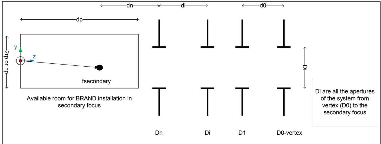
Figure 3. SECONDARY apertures and flat mirrors between the vertex hole and the secondary focus. It also shows the room available for the installation of BRAND receiver.
