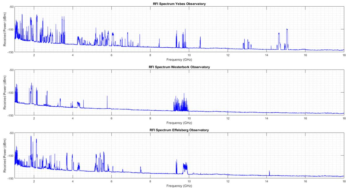
**Figure 13: Comparison of received power by an isotropic antenna.**
