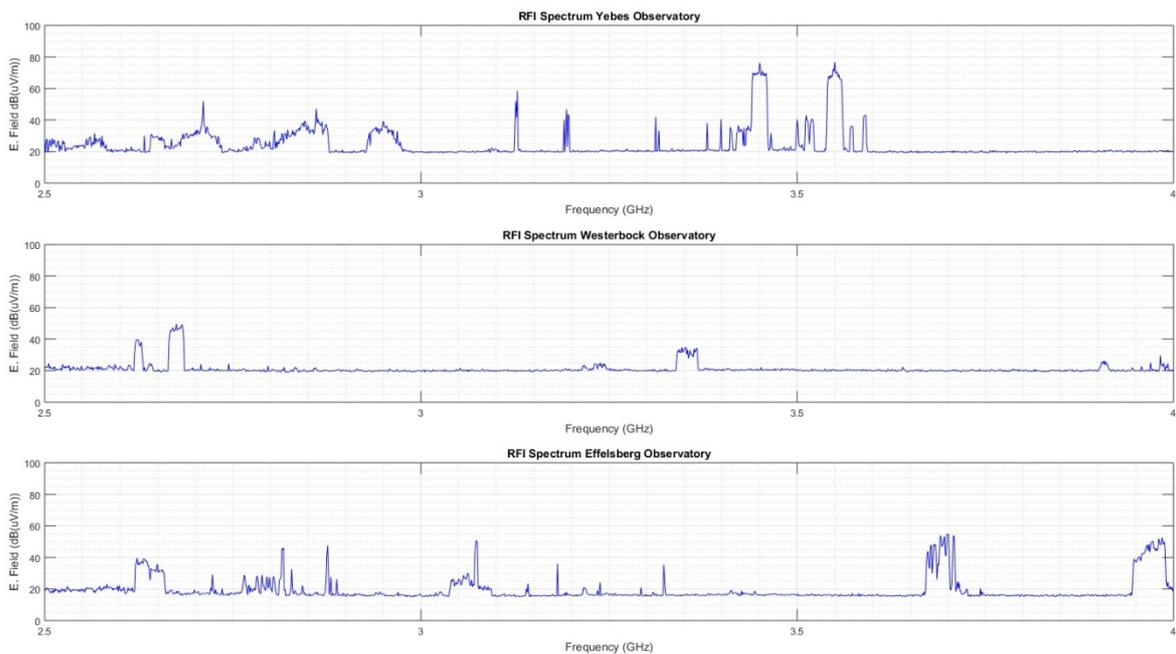
Figure 6: 2.5 - 4 GHz RFI spectrum comparison.
