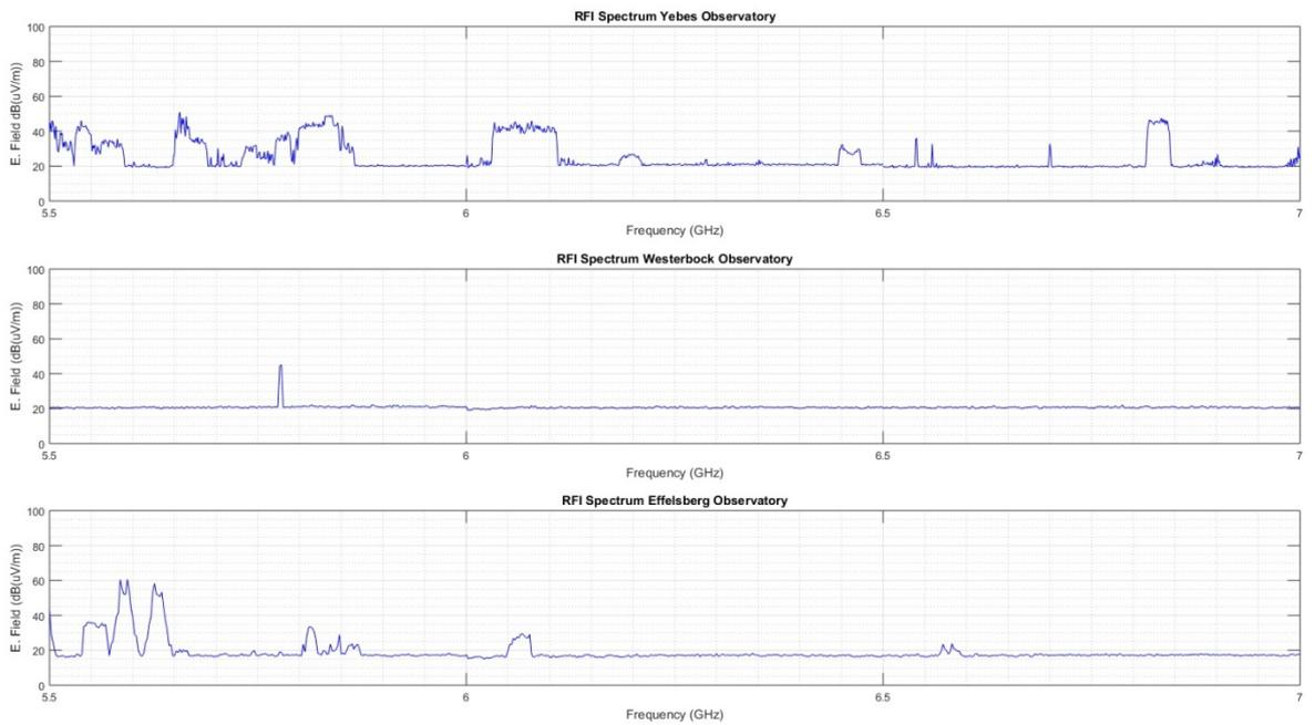
**Figure 8: 5.5 - 7 GHz RFI spectrum comparison.**
