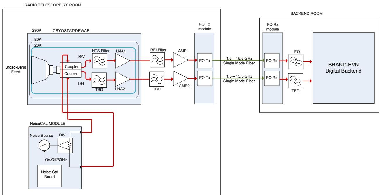
Figure 1: Broad-band receiver block diagram.
