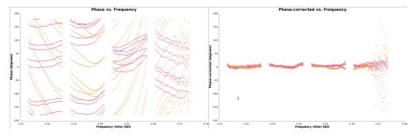
Fringe fitting results of EVN P band data with dispersive model – the algorithm correctly takes out the prominent 1/frequency curvature at the lowest bands and the linear terms at the higher frequencies.
