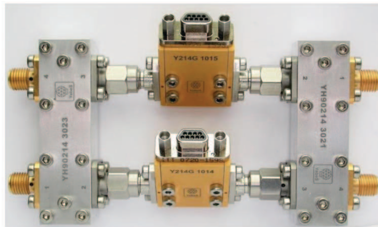
Fig. 3.3 Assembled balanced amplifier picture (without the matched loads). Length of the assembly excluding connectors is 82mm. Input is on the left and output on the right. Matched loads can be placed both on ports 1 or both on ports 4 of the hybrids in the picture, leaving the other couple of ports for input and output.
