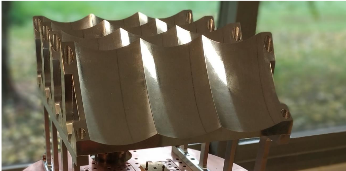
Fig. 30: View of the array of double face mirrors, located inside the cryostat
