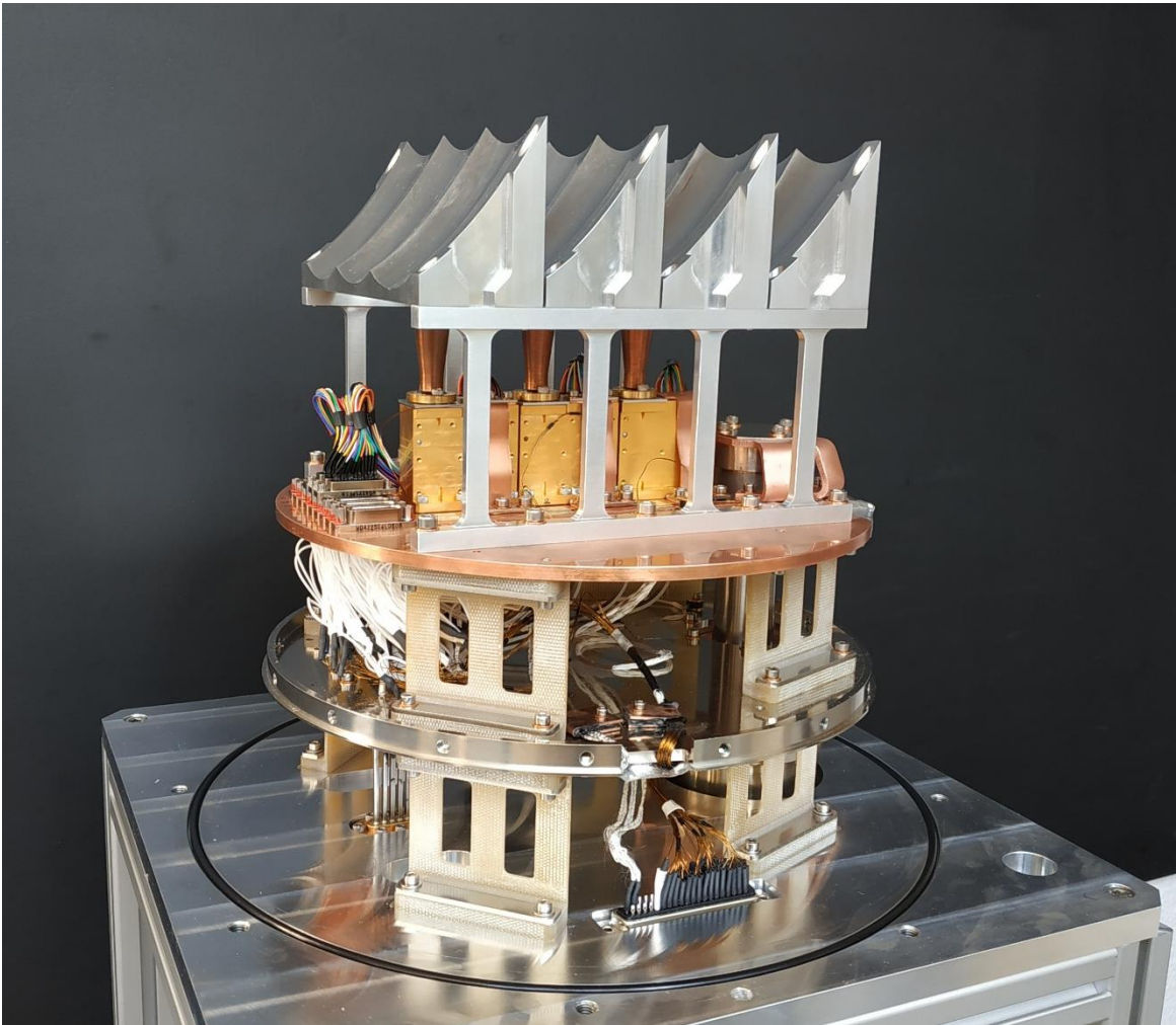
Fig. 40: WP5.1 Array demonstrator, fully assembled with three single-pixel modules installed.
