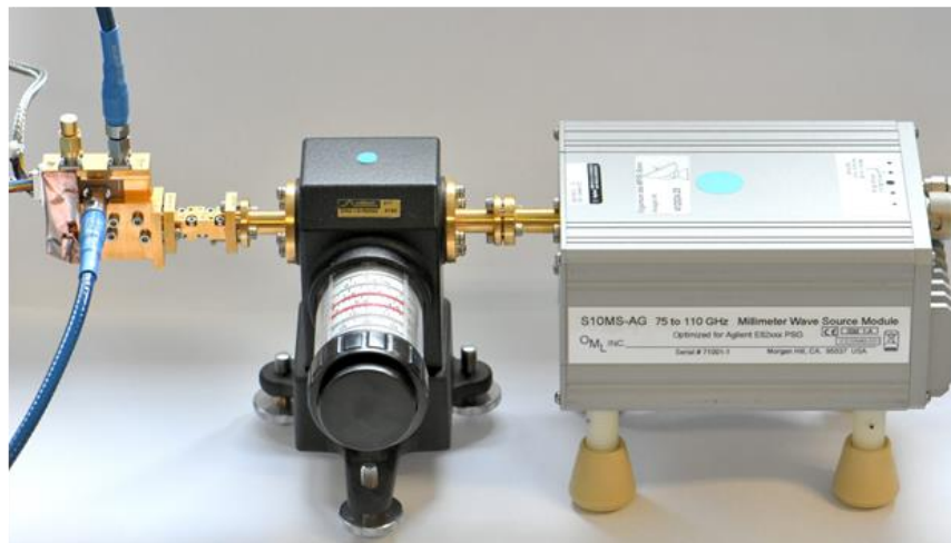
Fig. 22: Schematic and photograph of the test setup for the downconverter test-module.
