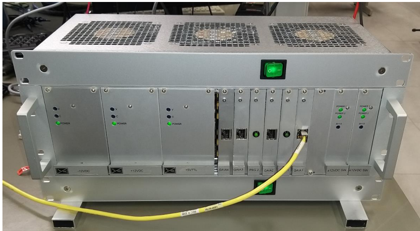
Fig. 38: Monitor and Control rack of the AETHRA WP1 receiver array demonstrator. The main rack (3U×19") incorporates four GAIA boards, two PSG boards, and five commercial power supplies. Two 1U cooling fans, one above and one below the main rack, are used to maintain a constant airflow through the electronics and avoid over heating of the PSG boards.
